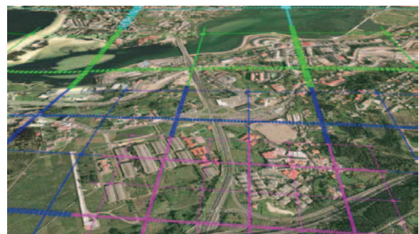
Figure 5: Virtual textures applied to the terrain. Levels of detail are shown using a color code.
