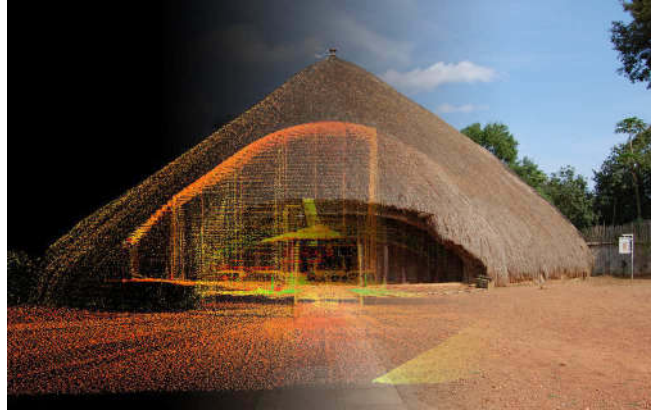
Figure 3.3: Example of a point-based rendering: photo overlaid atop laser scan data from a project held in early 2009 at Kasubi Tombs.
