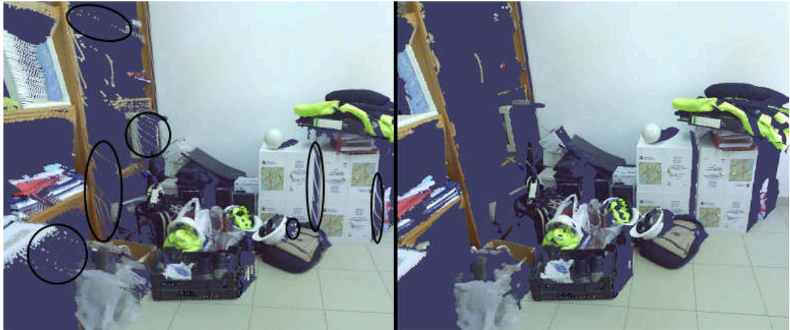
Figure 9.2: Original dataset without filtering applied, ellipses highlight outliers ( left ). Resulting dataset without outliers after filtering is applied ( right ).
