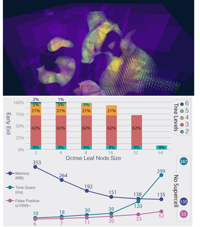
Fig. 9. Early-out with supercells. (Top) Octree nodes that exit tree traversal early are shown in purple. (Bottom) Efficiency of early-out with supercells for different octree leaf node sizes n^3 ( n = 2 to n = 64 ): Percentages of nodes exiting on a given tree level (root is level 0). With increasing node size, memory consumption decreases, but query times and false positive rates increase. Here, the sweet spot is around n = 16 .
