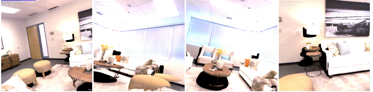
Figure 4: Frames extracted from browser-based exploration of Replica360 example scene. The frames are selected to show both successful viewpoints and remaining artifacts, including local ghosting, duplicated small objects, and unstable thin structures around clutter, plants, chairs, and table regions.
